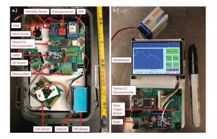
The measurement device houses the main circuit board. The CO and  $CO_2$  sensors are plumbed in line with a micropump and the particulate matter sensor is exposed to ambient air through a window on the side of the enclosure.
